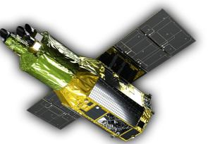
Xtend = XMA (X-ray Mirror Assembly) + SXI (Soft X-ray Imager)
